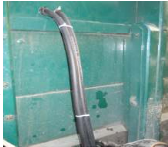
Image of the hoses leaving the truck bed, ziptied together for protection
