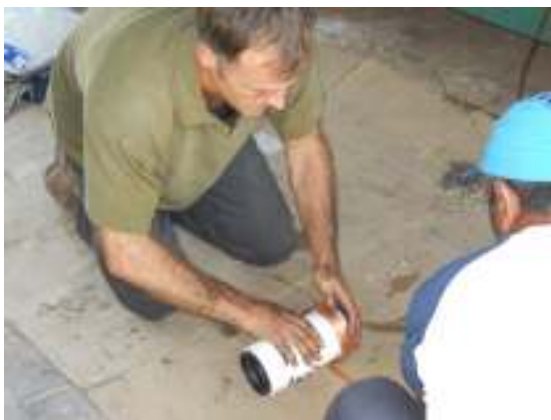
Above: Wrapping the copper hose around the filter Right: Shifting the coil to maximize contact between coil and filter
