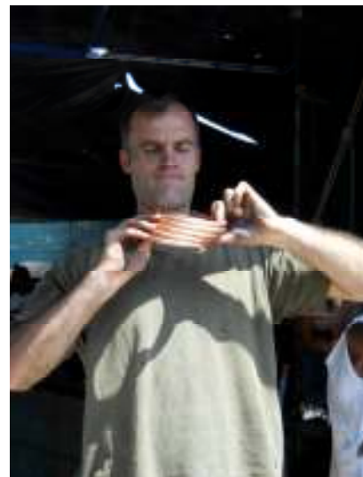
Above: Wrapping the copper hose around the filter Right: Shifting the coil to maximize contact between coil and filter
